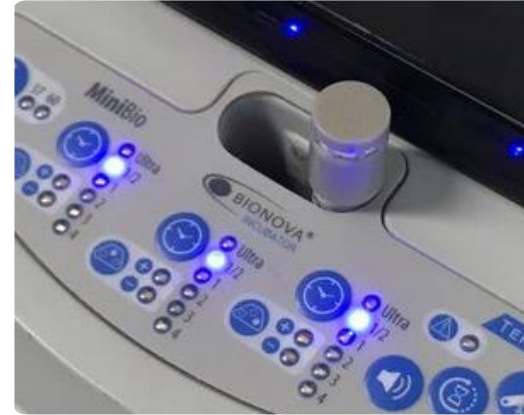
3. Put BI into Ampoule Crusher.
