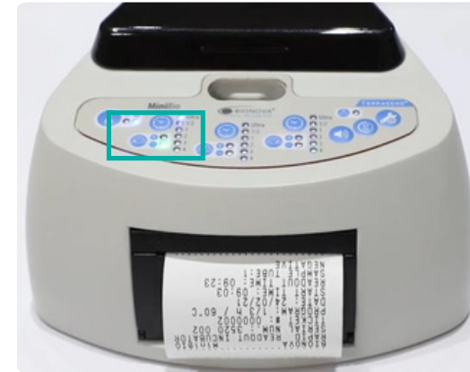
9. When the process is finished, a red or green light will appear, and the unit will print a ticket with the result.
