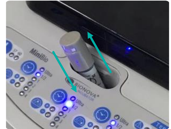
4. Push the BI to the left and back to break the BI.
