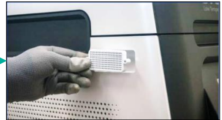
3. Remove the Ozone filter and replace it with new Ozone filter
