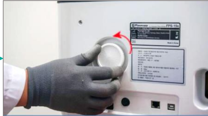
2. Remove the old HEPA filter by turning counterclockwise
