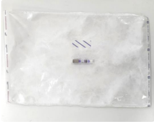
1. Put BI in Tyvek pouch with CI strip and run the cycle.
